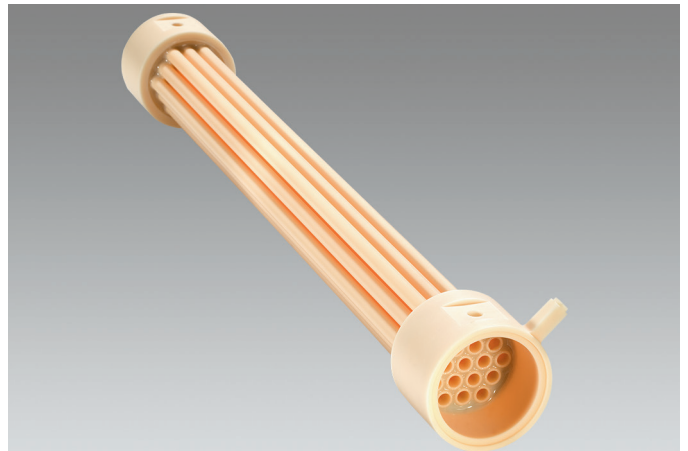
Fig. 9: Glass-brazed ozone generator made of aluminium oxide FRIALIT F99.7
