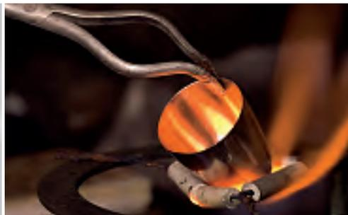
Ögussa makes a number of accessories to enable you to expertly handle crucibles and dishes in the laboratory, such as crucible tongs made of chromium nickel steel in various lengths, which are fitted with platinum shoes or solid platinum tips. As a special design we offer platinum shoes which extend up to the swivel-joint. Tweezers can also be supplied with platinum shoes or solid platinum tips.
