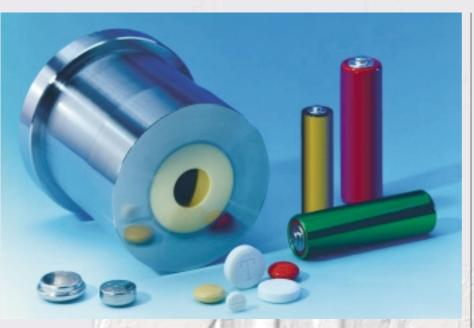
Fig. 2: Compression moulds for the high-pressure compaction of powders into solid shapes. K (?) (Works photo Friatec AG Division Frialit-Degussit)
